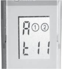
Following the start-up phase, the top left of the display shows the operating mode A. The loop symbol(s) are shown adjacent to that and, underneath, the set basic functions. At the bottom left, a "t" displays whether or not a time function has been programmed. Now, the function can be checked by activating the loop with the intended object. If the loop is activated, the output relay must switch on or off depending on the selected function.
